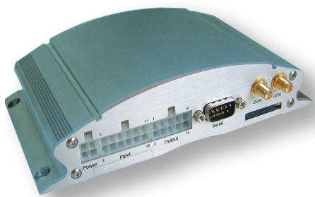
Fig. 3. The X8 AVL system
